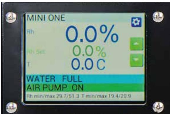
Ambient gallery air is filtered for pollutants and drawn into the unit. This air is pressurized and directed through a proprietary mechanism that adjusts the relative humidity to the pre-set value. This air is directed through a small flexible tube to an input port in the showcase. Air flow to the enclosure is constant, and in normal applications the air is delivered only at the preset relative humidity.
