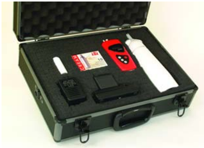
Figure 2. Air exchange measurement equipment case includes gas detector PM3010, Cream whipper and N 2 O chargers, external battery and charger. Portable computer also required for analysing data
