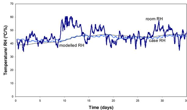
Figure 4. Apsley House cases. Modelled and measured RH. The model correctly describes the general trend, but underestimates short term RH variations.
